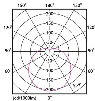
Light Distribution Diagram - Ess LEDBulb 8-60W E27 3000K 4PF/6 MX
